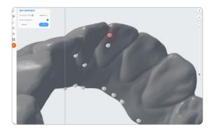
**Tip**: To quickly remove multiple support points from anatomy click and drag and release across the points you want to remove and hit the delete key on your keyboard.
