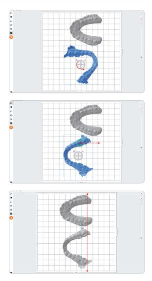
**Tip**: When setting up multiple models you can quickly get them into position by rotating and overlapping the parts. The corner or edge of the build platform can be helpful as a stop.
