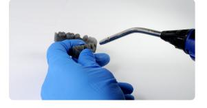
Inspect printed parts to ensure that parts are clean and dry.
