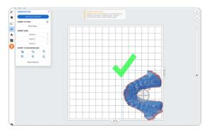
Once the models are positioned, view the build from the side. Use the view tools on the top right of PreForm as shown.
