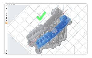
**Tip**: For parts printed directly on the build platform, when positioning models so that the pry point is facing toward the outside of the build platform. This will simplify part removal once printed.
