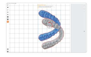
**To rotate the part** while it is selected, click-anddrag the outer edge of the orientation sphere.
