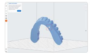
Typically, **models printed directly to the platform do not require any support structures** or additional steps.
