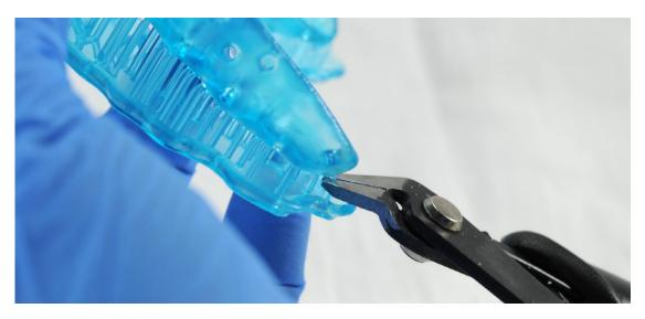
Remove supports using a cutting disk and handpiece, or other part removal tool.
