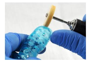
**Note:** Lathes with rag or felt wheels, pumice, and high shine compound make the process quick and easy.
