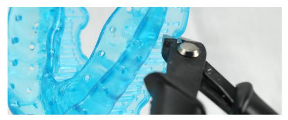
Removing supports should leave a small positive feature.
