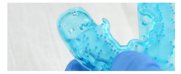
Inspect the custom tray. Discard and reprint the part if any cracks are detected.
