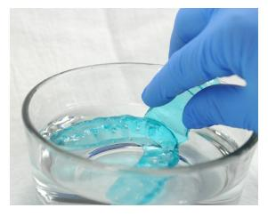
**Note:** Do not leave the part in the alcohol solution for longer than 5 minutes.
