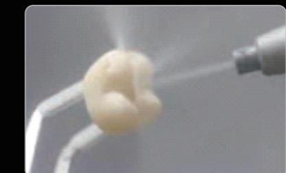
Sandblast under 2-2.5Bar with 50µm Al<sub>2</sub>O<sub>3</sub> grit, Polish the crown if applicable.
